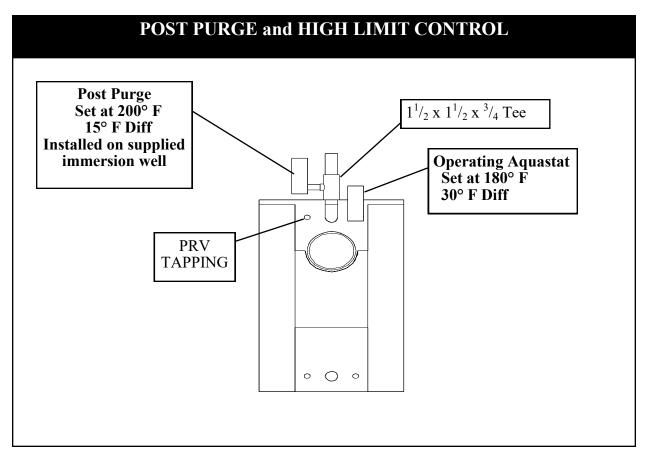
The post purge control (L4006A) must be mounted on the immersion well in  $1^{1}/_{2}$  x  $1^{-1}/_{2}$  x  $3^{-1}/_{4}$  tee supplied with DVH Trim Kit.
