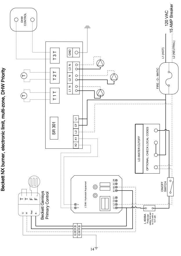
Note 2: All wiring must be done in accordance with applicable state, local and national codes. Use only copper conductors.
